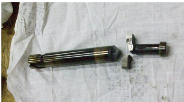
Fig.1: Broken Plunger Flange
