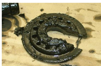
Fig.2: Sticking and Contamination of FO Injection Pump
