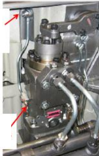
Fig.3: Lubricating Pipe of Pinion Rack
